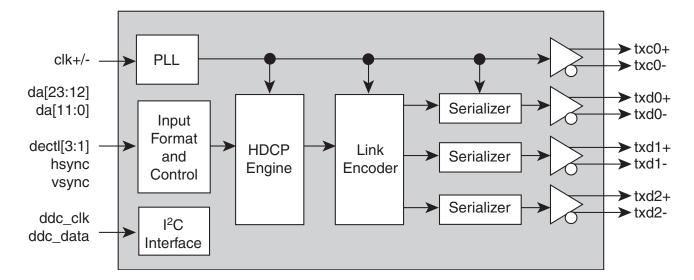
The BCM7501 is part of Broadcom's family of video display products, and is a full rate, single link, DVI 1.0-compliant transmitter with HDCP content protection. The BCM7501 transmits digital video from a digital host such as a PC graphics card, set-top box, or DVD to a display such as an HDTV, flat panel display, or digital CRT. The DVI interface is uncompressed, low-cost, and digitally protected, making it ideal for Consumer Electronics (CE) applications.
