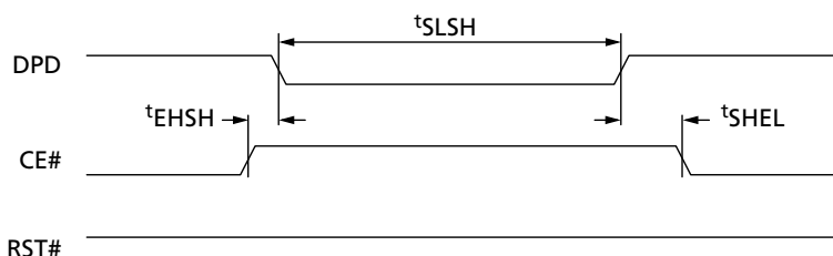
Figure 18: Deep Power-Down Operation Timing
