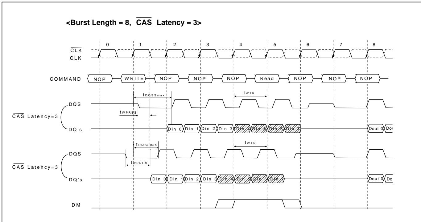
The following functionality established how a Read command may interrupt a Write burst and which input data is not written into the memory.
