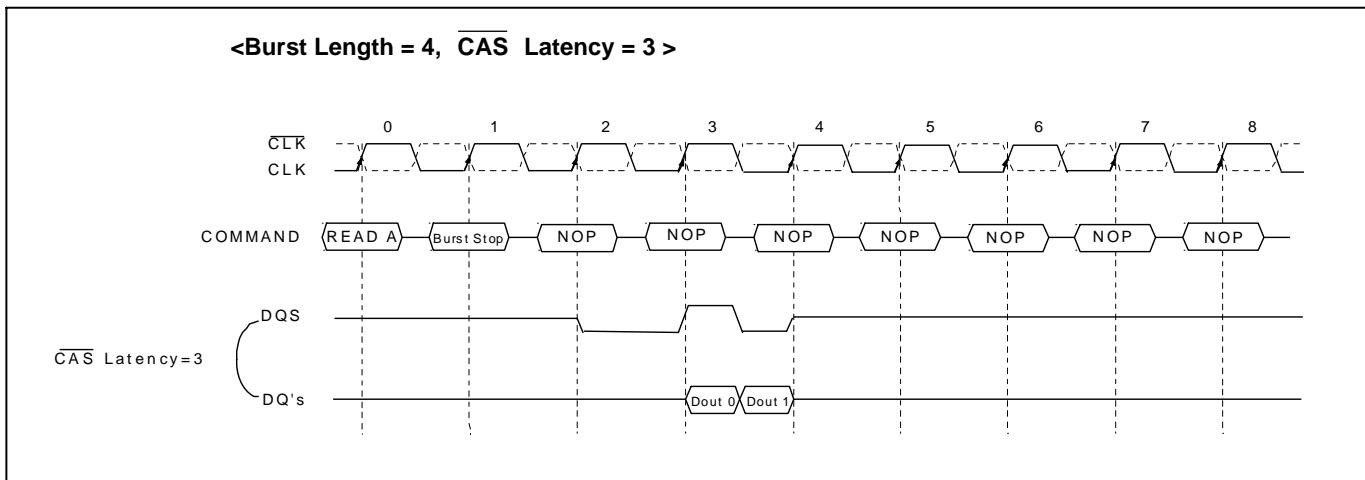
The Burst Stop command is a mandatory feature for DDR SDRAMs. The following functionality is required.
