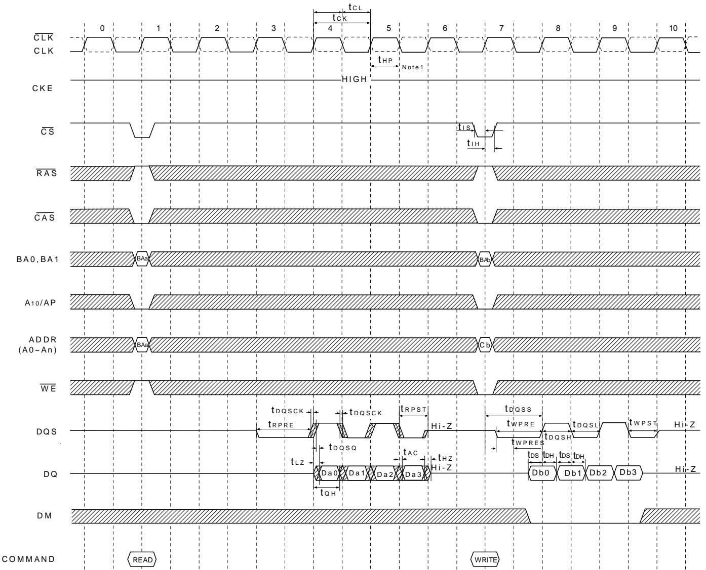
Note 1.  $t_{HP}$  is lesser of  $t_{CL}$  or  $t_{CH}$  clock transition collectively when a bank is active.
