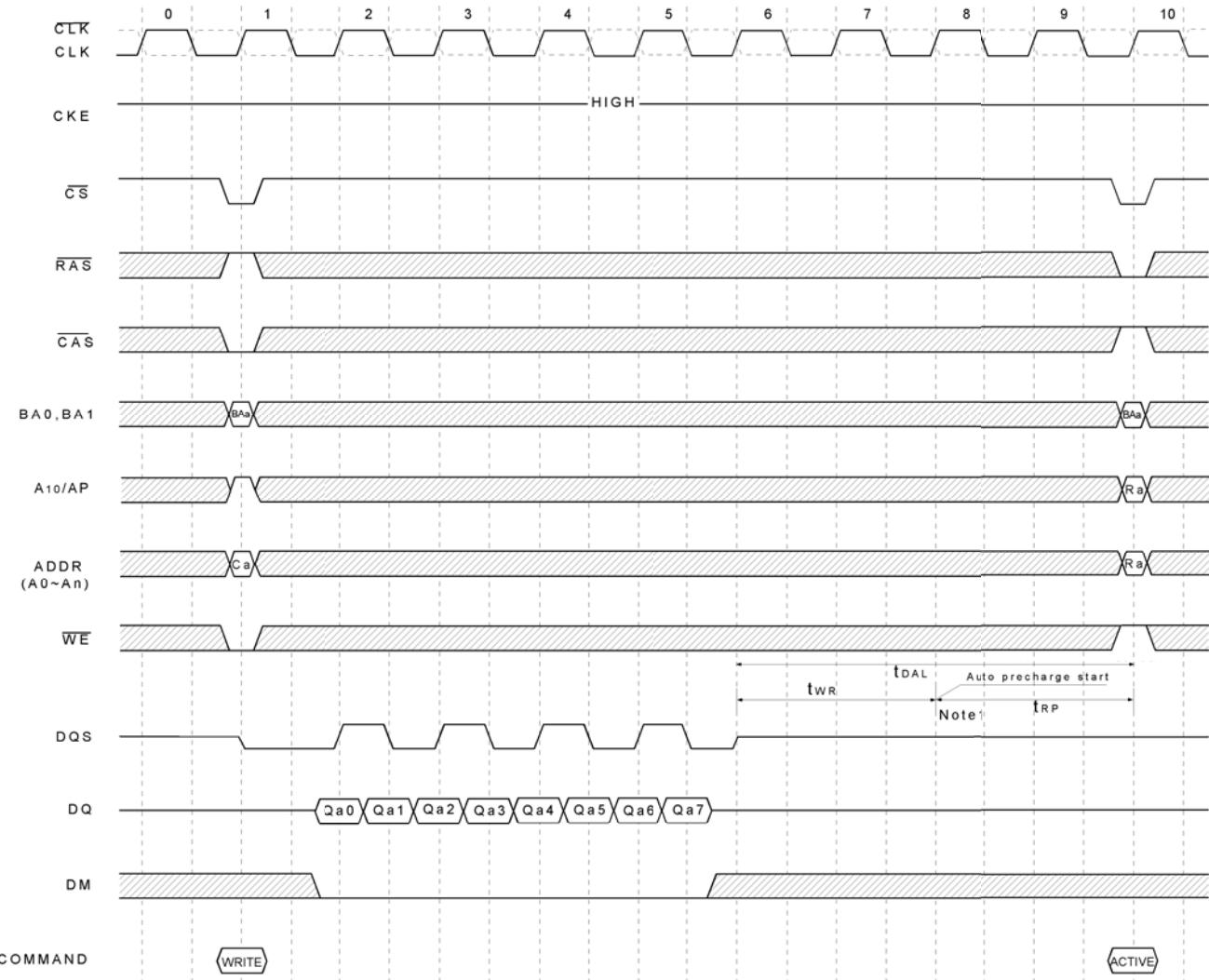
Note 1. The row active command of the precharge bank can be issued after  $t_{RP}$  from this point.
