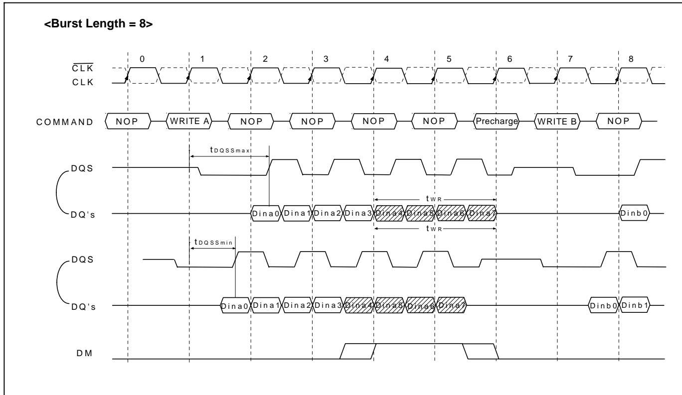
Precharge timing for Write operations in DRAMs requires enough time to allow "Write recovery" which is the time required by a DRAM core to properly store a full "0" or "1" level before a Precharge operation. For DDR SDRAM, a timing parameter,  $t_{WR}$ , is used to indicate the required of time between the last valid write operation and a Precharge command to the same bank.
