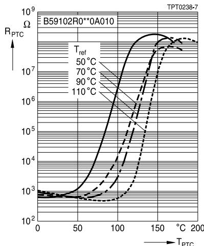
PTC resistance  $R_{PTC}$  versusPTC temperature  $T_{PTC}$
