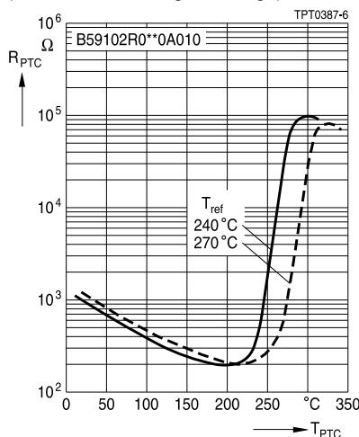
PTC resistance  $R_{PTC}$  versusPTC temperature  $T_{PTC}$
