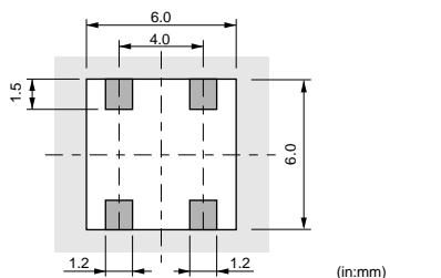
The solder resist should be printed except for the land pattern on the P.C.B..
