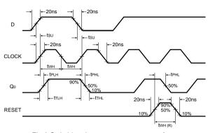
Fig.2 Switching time measurement waveform
