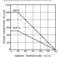
Fig.3 Power dissipation vs. ambient temperature
