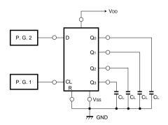
Fig.1 Switching characteristics measurement circuit
