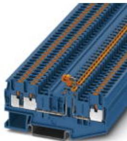
Knife disconnect terminal block, Connection type: Push-in connection, Cross section: 0.14 mm<sup>2</sup> - 4 mm<sup>2</sup>, AWG: 26 - 12, Nominal current: 16 A, Nominal voltage: 400 V, Length: 81.9 mm, Width: 5.2 mm, Color: blue, Assembly: NS 35/7,5, NS 35/15
