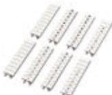
Zack marker strip, Strip, white, labeled, Printed horizontally: Consecutive numbers 1 - 10, 11 - 20, etc. up to 491 - 500, Mounting type: Snap into tall marker groove, for terminal block width: 5.2 mm, Lettering field: 5.15 x 10.5 mm
