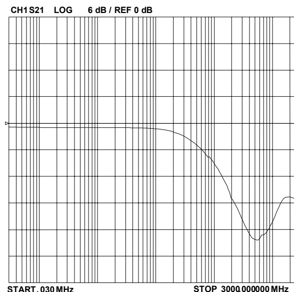
Figure 2 - Typical Insertion Loss S21
