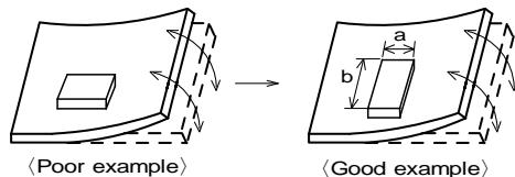
Products shall be located in the sideways direction (Length: a**a**b) to the mechanical stress.
