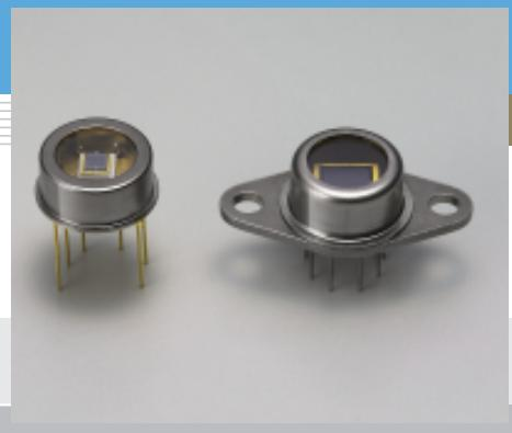
S2592/S3477 series sensors combine a UV to near infrared Si photodiode with a thermoelectric cooler. A thermistor is also included in the same package to sense the Si photodiode chip temperature. This allows stable operation over long periods of time, making these sensors suitable for low-light-level detection where a high S/N is required.
