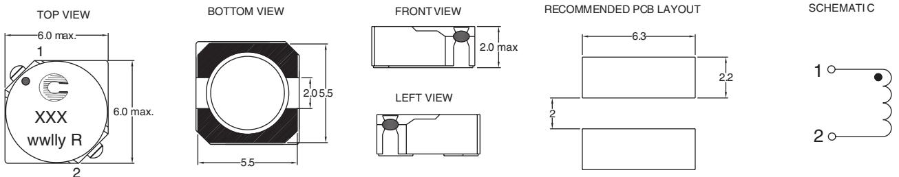
Dimensions are in millimeters.
