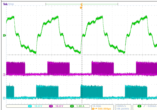
Figure 11. Stepper Control, Full Stepping, 12V
