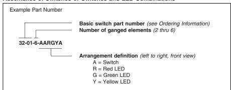
Example part number describes a stack of 6 elements consisting of two switches, a red LED, a green LED, a switch and a yellow LED. Shorter stacks will have fewer letters in the arrangement definition. Contact Grayhill for stacks of more than six elements.
