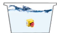
IP67: Submersion to one meter for 30 minutes.
