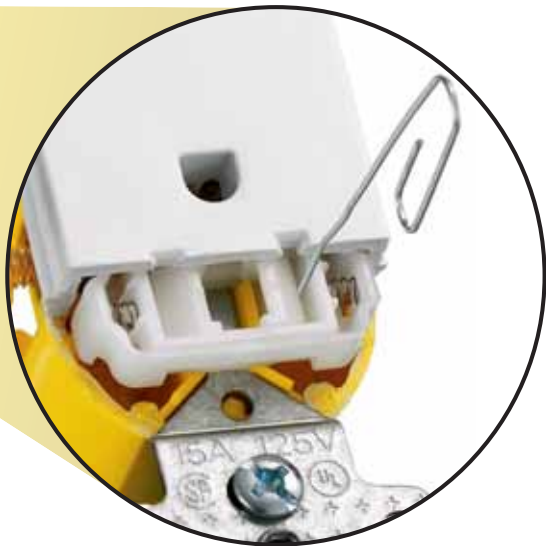
SAFETY IN ACTION Spring-loaded shutters lock out a single object, effectively blocking entry to the contacts.
