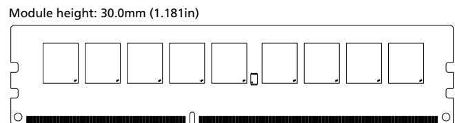
Figure 2: 240-Pin UDIMM (MO-269 R/C D1) PCBs 1483 &1568
