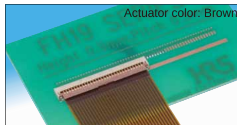
FH19SC – FPC/FFC thickness: 0.3 \pm 0.03 mm
