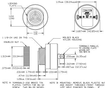
NOTE A: TERMINALS-.032 BRASS TIN PLATED, TAPPED FOR #6-32 SCREW. TWO #6-32 NICKEL PLATED BRASS SCREWS INCLUDED. WILL ACCEPT 1/4' QUICK CONNECT.
