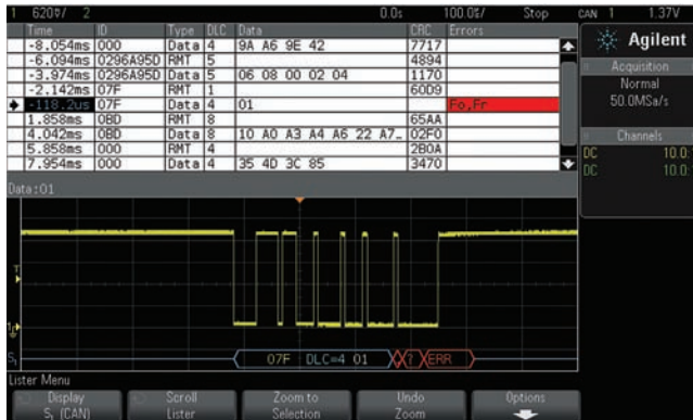
Figure 1: Hardware-based decoding quickly reveals serial communication errors.
