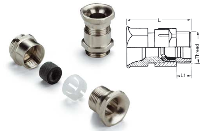
Cable gland with bending protection and internal strain relief. Without external strain relief clamp. Clamping profile made of Hostaform C.
