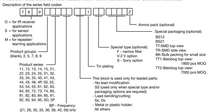
Example: TSOP1236TB1 = receiver with  $f_0$  = 36 kHz, bent in a top view holder, and solder plated leads
