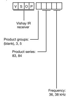
Example: VSOP38336 = receiver chip with  $f_0 = 36 \text{ kHz}$
