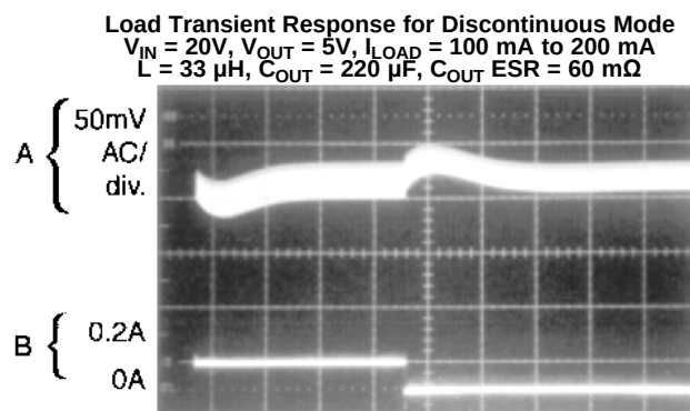
Figure 23. Horizontal Time Base: 2 \mu\text{s}/\text{div} .
