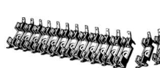
One piece self-aligning fuse clip/terminal design. Breakaway poles for easier stocking and ordering. Protective pole barriers surround each clip to provide greater protection against clip damage and electrical shock. Low profile design. UL recognized and CSA certified at 300 V. Molded of glass reinforced thermoplastic. UL 94VO flammability rating. Clip/Terminal: High tensile spring brass, electro-tin plated. Standard gray color.
