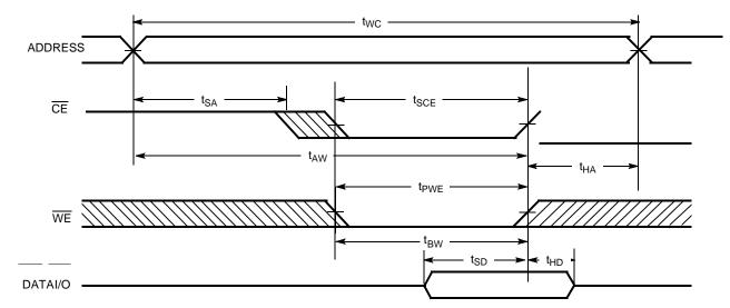
Write Cycle No. 2 ( $\overline{\text{WE}}$  Controlled,  $\overline{\text{OE}}$  LOW)[16, 17, 18]
