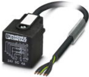
Sensor/Actuator cable, 5-position, PUR halogen-free, Black RAL 9005, Free cable end, on AD valve plug (pressure switch), with 2 LEDs, Cable length: 1.5 m
