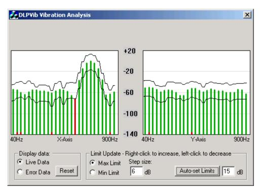
This program is designed to monitor both channels of the accelerometer and graphically display frequency and amplitude data proportional to the vibration. Limits can be set such that an error indication is made when any frequency component rises or falls out of the limits.
