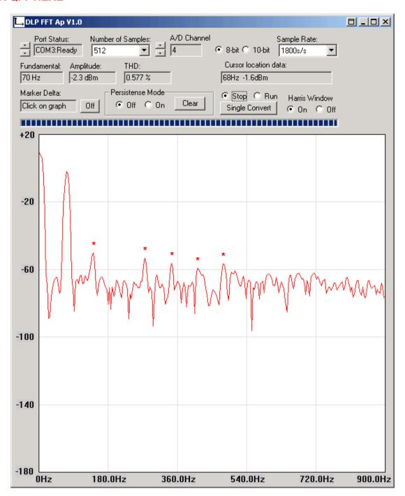
This program is designed to acquire AC signal data from any of the seven analog inputs on the DLP-TILT, then calculate and display the FFT of the signal and provide some basic analysis. Numerous program settings are possible including setting the COM port, A/D channel on the microcontroller, sample rate, number of samples, and a continuous run mode.
