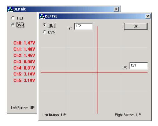
This program is designed to both demonstrate the tilt feature of the accelerometer and present the acquired voltages from each of the seven analog inputs.
