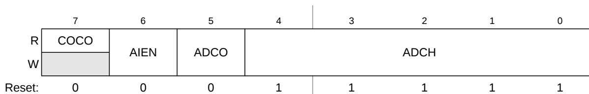
Figure 10-3. Status and Control Register (ADCSC1)
