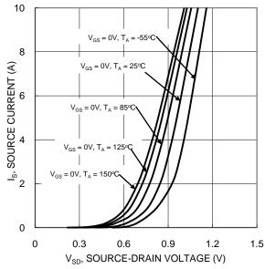
Figure 9 Diode Forward Voltage vs. Current
