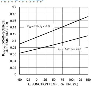
Figure 7 On-Resistance Variation with Temperature
