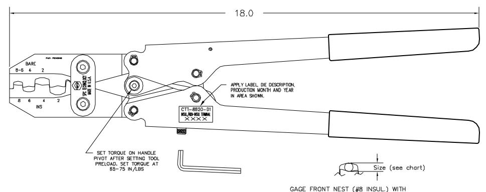
HEAT TREATED COMPONENTS BLACK OXIDED JAW ASSEMBLY BLACK OXIDED HANDLE ASSEMBLY BLACK TEXTURED PLASTISOL GRIPS TOOL PRELOAD SET TO 11"-11 7/16" AT END OF HANDLES WITH GRIPS ON
