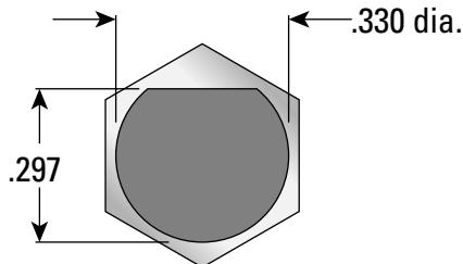
Flat of mounting surface is aligned with body hex as shown.
