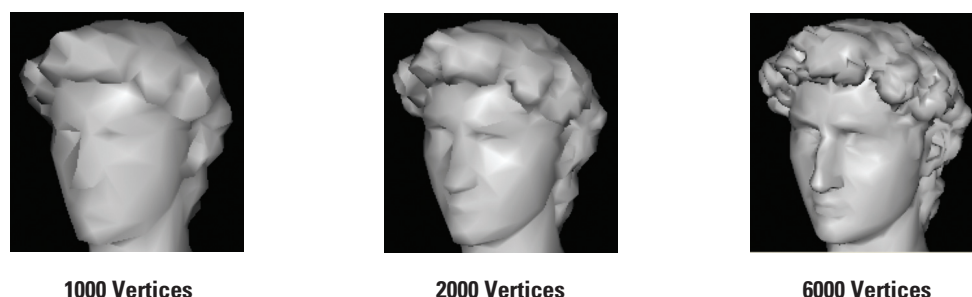
Figure 4. Example of a vertex-shaded 3D model rendered with increasing tessellation.
