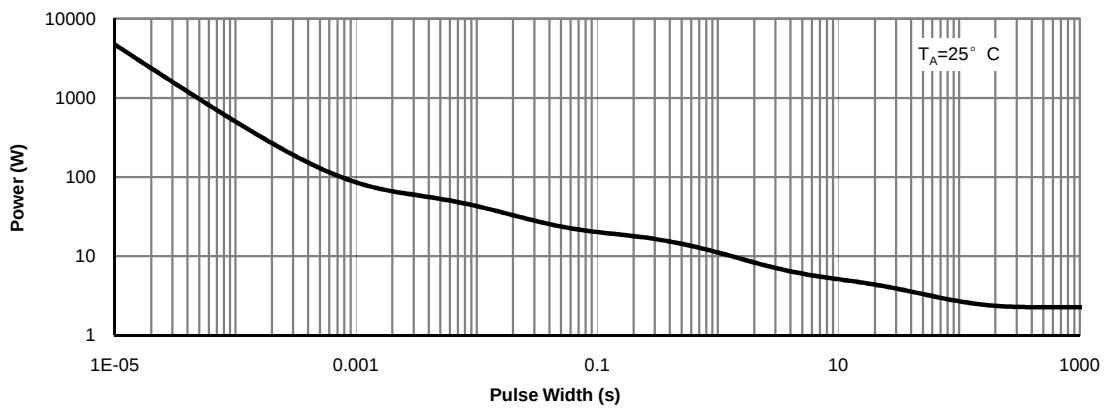
Figure 14: Single Pulse Power Rating Junction-to-Ambient (Note H)
