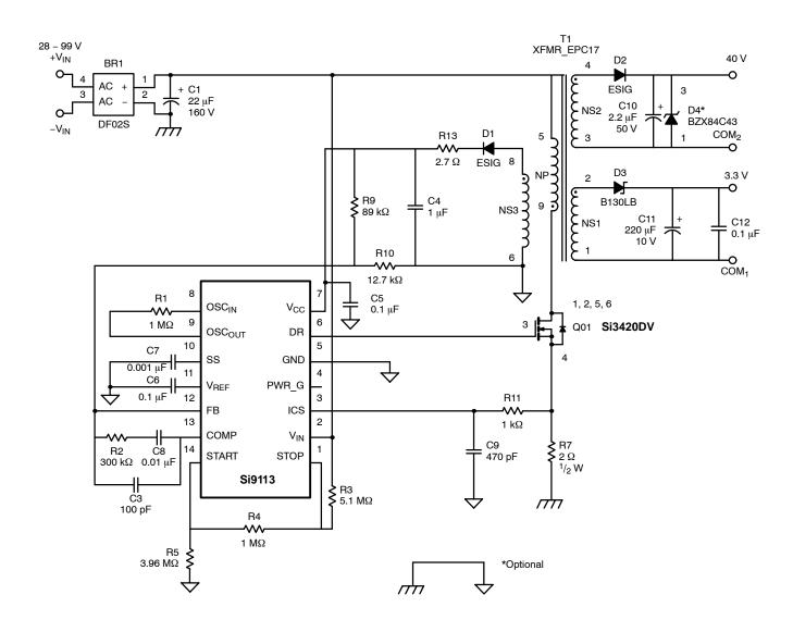
FIGURE 3. Dual Output Flyback Converter with Moderately Regulated Outputs (As used on Demo Board DB-2)
