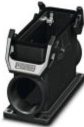
Box mounting bases B24, with double locking latch, material: PA, cable outlets: 2, lateral, height: 84 mm, cable gland: none, gland: no, 2x M25, Standard, including 2x reducing adapter
