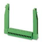
Direct plug-in block, nominal current: 12 A, rated voltage (III/2): 320 V, nominal cross section: 2.5 mm², number of positions: 21, pitch: 5.08 mm, connection method: Screw connection with tension sleeve, color: green, contact surface: Tin, mounting: Direct mounting
