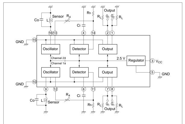
Notes: R<sub>4</sub>: Sensing distance adjustment resistor
