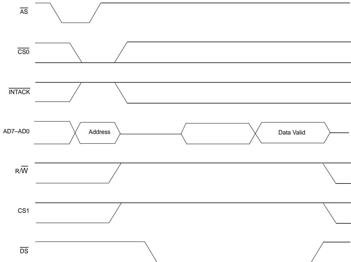
Figure 24. Read Cycle Timing
