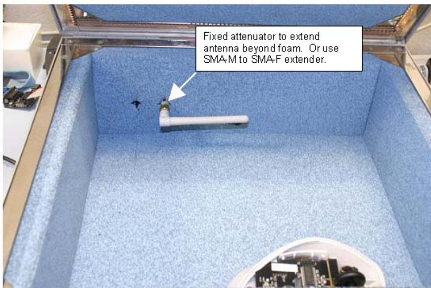
Figure 2-1. Fixed Antenna Mounting Example
