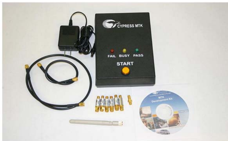
Figure 1-1. Manufacturing Test Contents
