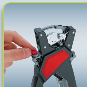
Adjust cross section
