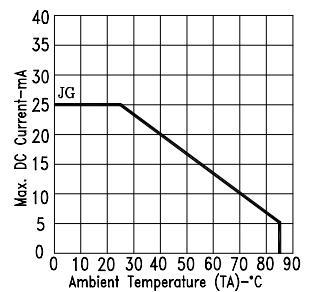
Fig 5. MAX. ALLOWABLE DC CURRENT VS. AMBIENT TEMPERATURE.
