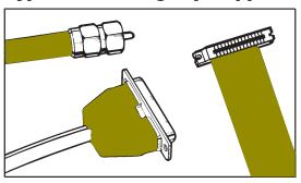
3M<sup>™</sup>Shielding Tapes are used as ground planes or shields for electronic cables and connectors. The tape is bonded to the cable's conductive sheath and to the metallic lip of the connector to provide a complete shield from end to end.
