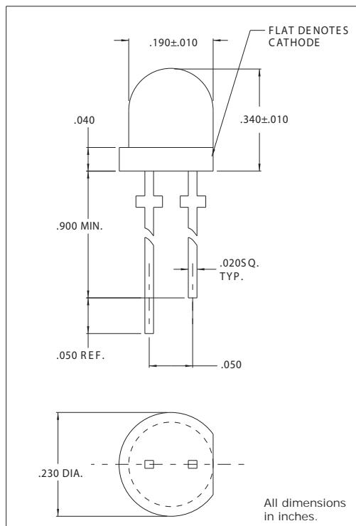
The Ultrabright HLMP3X50 series are direct pin for pin replacements for Hewlett Packard's HLMP3X50 series. These LED lamps provide a very narrow viewing angle in a clear tinted non-diffused package and are excellent for small area backlighting. A pale tint aids in identification. The High Efficiency Red and Yellow lamps are produced with GaAsP/GaP and the High Efficiency Green lamp is produced with GaP/GaP. All feature an 80 mcd minimum luminous intensity.
