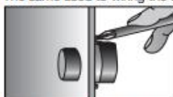
The holder will be secured at the back by two screws or nuts.
