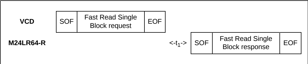
Figure 67. Fast Read Single Block frame exchange between VCD and M24LR64-R
