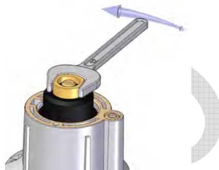
Figure 24: Adjusting flow rate.
