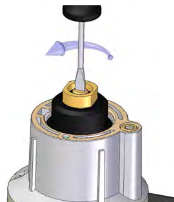
Figure 25: Adjusting step pressure.
