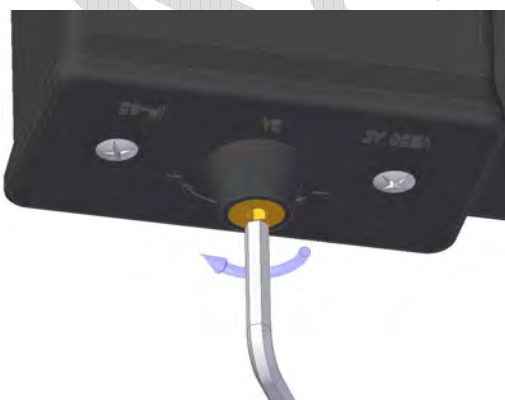
Figure 24: CPI switch adjustment
