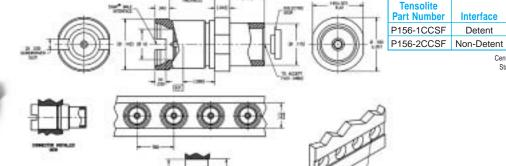
Center conductor is captivated. Standard finish is passivated.
