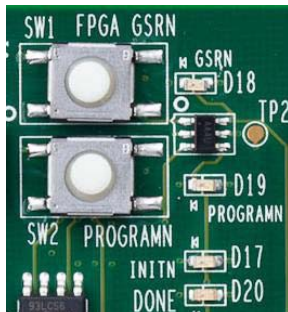
Figure 3. LatticeECP3 Status LEDs and Push-button Controls
