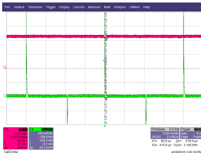
Figure 37 – 230 VAC, 5° Phase. Upper: V_{OUT} , 10 V / div. Lower: I_{IN} , 0.1 A / div., 5 ms / div.
