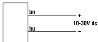
Emitters with Attached Cable
