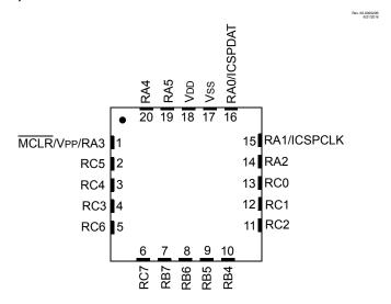
Note: It is recommended that the exposed bottom pad be connected to V<sub>SS</sub>.
