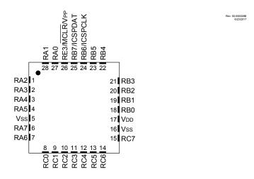
Note: It is recommended that the exposed bottom pad be connected to  $V_{SS}$ .
