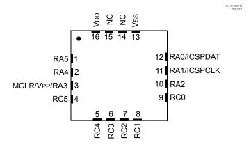
Note: It is recommended that the exposed bottom pad be connected to V<sub>SS</sub>.
